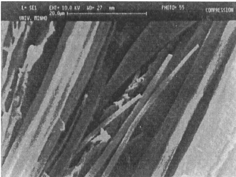
FIGURE 14 SEM micrograph of the MFC after compression molding.
